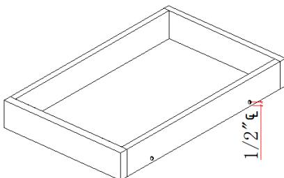
Step2: Mount short parts of (E) on each side of (A), using 7-screws(4pcs).
