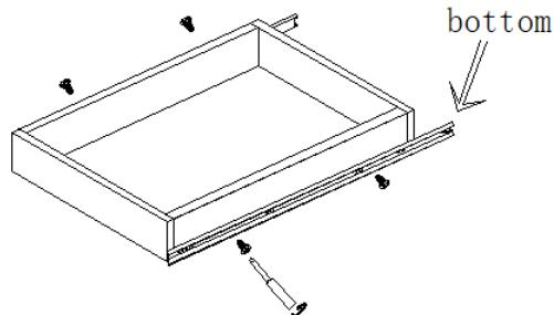
Step3: Must Predrill the Pilot Hole (1/4" Depth or less) on Face Frame of Cabinet. (Recommend 1/8" drill bit)
