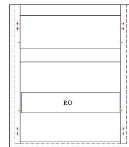
Step4: Mount long parts of (E) on Face Frame, using 7-screws(2pcs).
