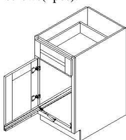
Step5: Mount Rear Brackets of (E) on Back Panel, using 7-screws(4pcs).
